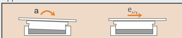
Fig. 1. Pot bearing under rotation and movement load
