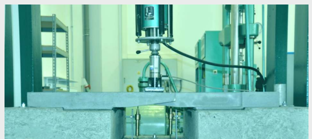
Picture 2. B2P finger expansion joint during the dynamic test
