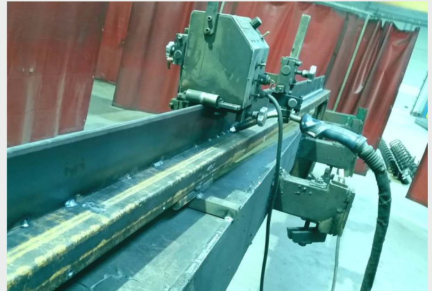
Picture 3. Welding steel profiles
